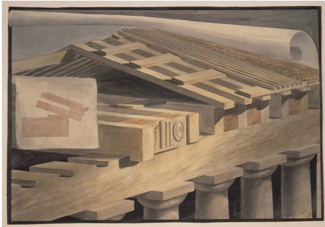
Royal Academy lecture drawing prepared by one of Soane's pupils in 1807, showing the origin of the Doric order
